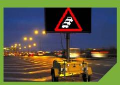
mobile variable message signs if required. Slow moving traffic is detected using crowd sourced data, which in turn activates 'Queue Ahead!' on one or more variable message signs.
