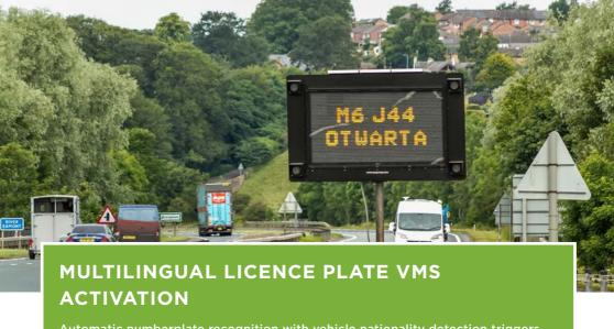
Automatic numberplate recognition with vehicle nationality detection triggers multilingual language warning messages. Using the latest ANPR cameras, VPS can detect the nationality of vehicles that pass the camera and display a translated message on the mobile variable message signs ahead, keeping all our international road users safe and fully informed of any hazards.
